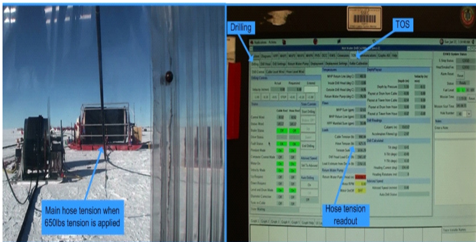
Figure 9.39 Hose tension at 650lbs load and screen where hose tension is displayed
