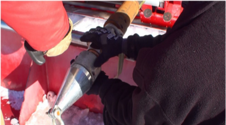
Figure 9.6 Tapered end cap fitted to end of main hose
