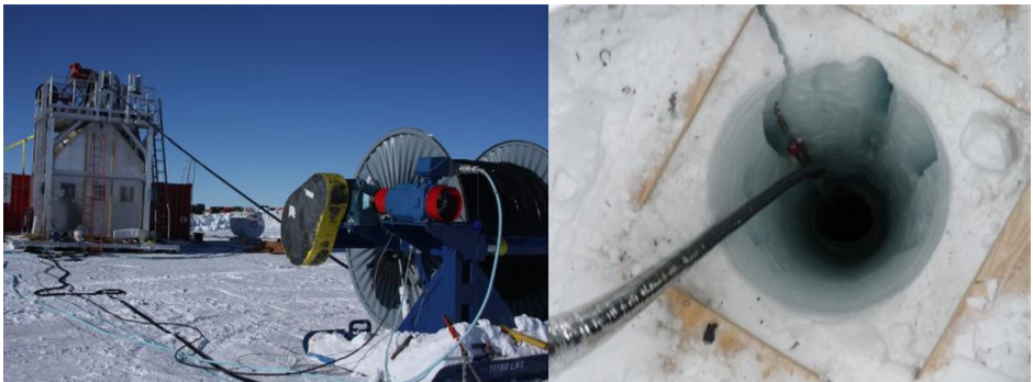
Figure 12.1 Deployment cable shown anchored to deadman
