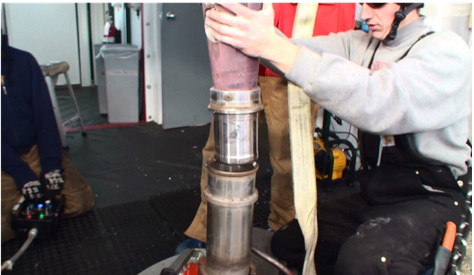
Figure 9.22 Drill head about to be mated with the weight stack.
