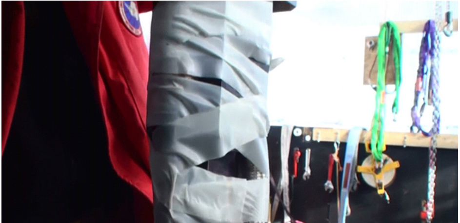
Figure 9.33 Tape applied to drill head adaptor hose and connector.
