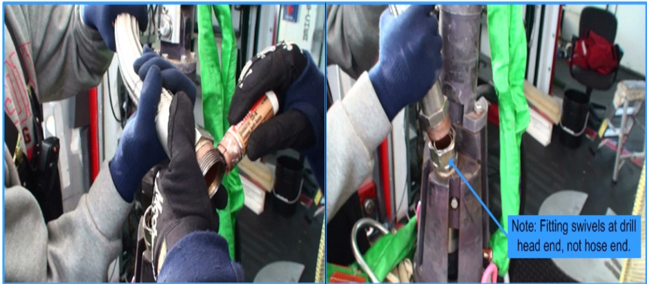
Figure 9.29 Preparing and connecting adaptor hose to drill head
