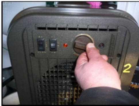
Figure 14.2 Heater thermostat control
