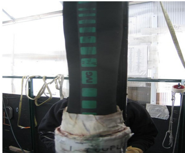
Figure 2.116 Axial fibres breaking under excess load, resulting in hose necking
