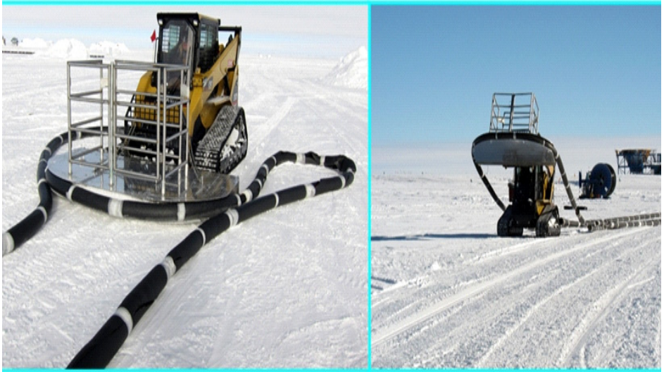
Figure 11.6 Hose relocator connected to 827 loader relocating hose to new hole.
