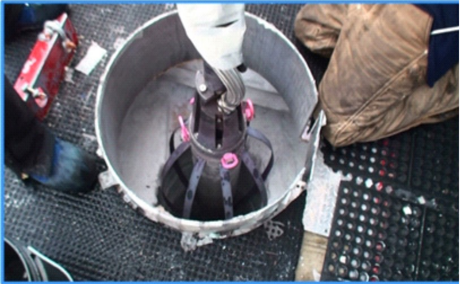
Figure 9.40 Drill Head position prior to "zeroing" payouts
