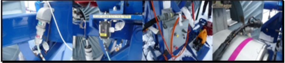
Figure 12.8 Deployment reel cables (drum, brake, octopus and sensor cables)
