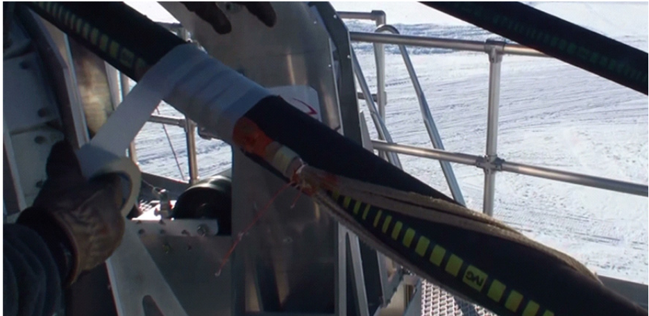
Figure 9.38 Taping main hose Yale grip anchor to hose
