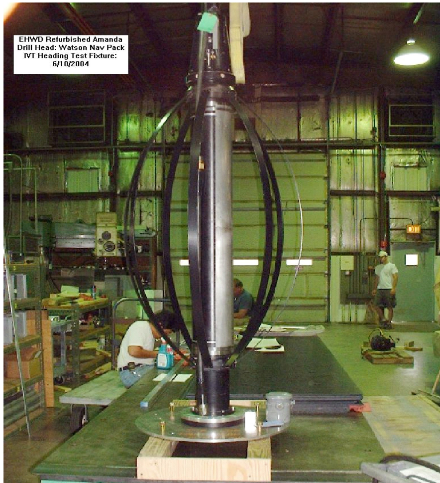
Figure 2.130 Drill head on test stand for testing and calibration
