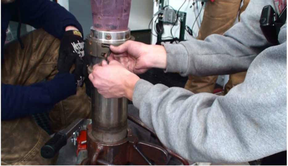
Figure 9.23 Drill head clamp collar attaching drill head to weight stack
