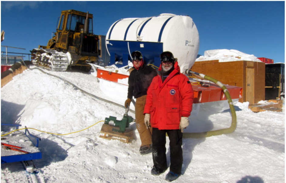
Figure 6.18 Seed water delivery tank tilted towards hose and delivering water
