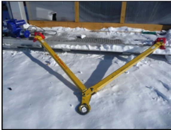
Figure 12.23 Tow bar attached to tower in preparation for move
