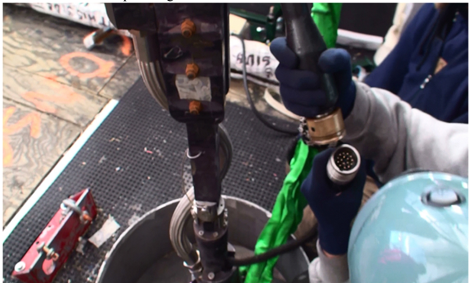
Figure 9.30 Attaching the drill cable to the drill head
