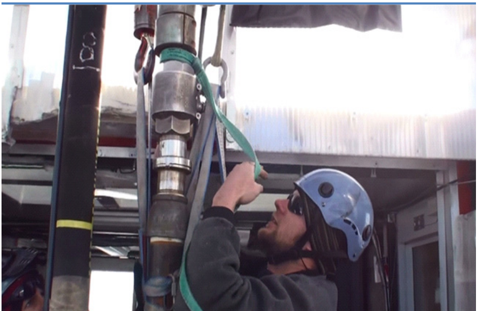
Figure 9.55 Attaching return water hose to pump.
