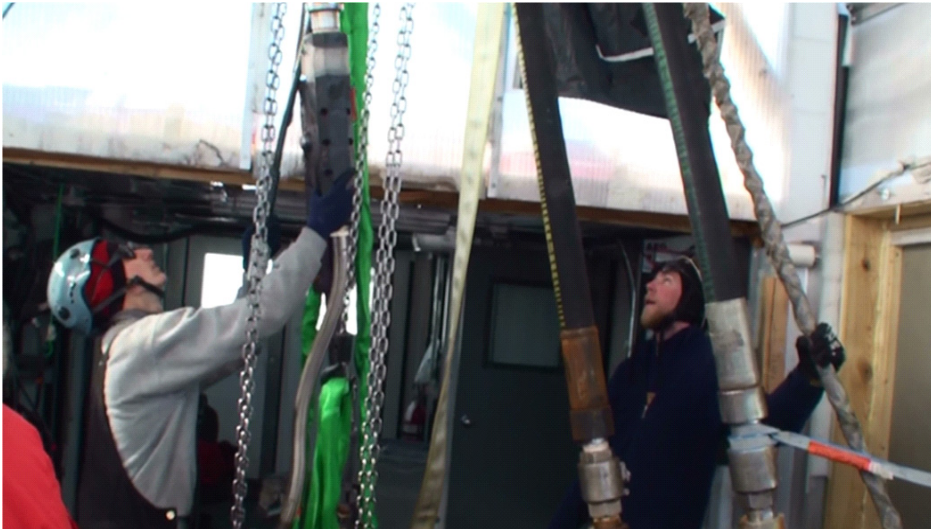
Figure 9.28 Drill head being raised by drill cable reel
