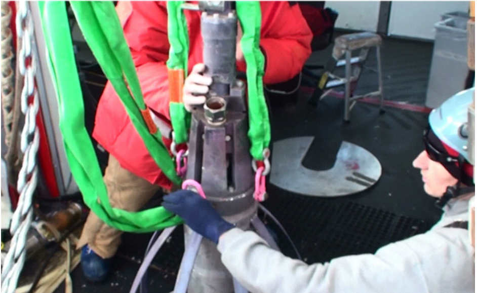
Figure 9.25 Drill head positioned at comfortable working distance above tower floor.
