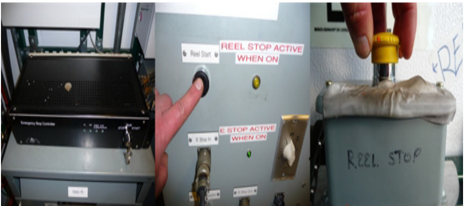
Figure 14.17 E-stop controller, reel start and slap button reset
