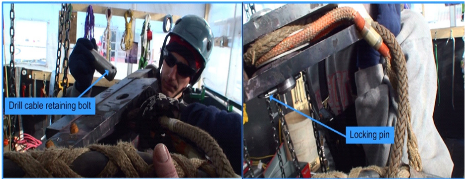
Figure 9.27 Connecting drill cable to drill head hanger
