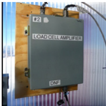
Figure 14.15 Cable needs to be reconnected to bottom of load cell amplifier box
