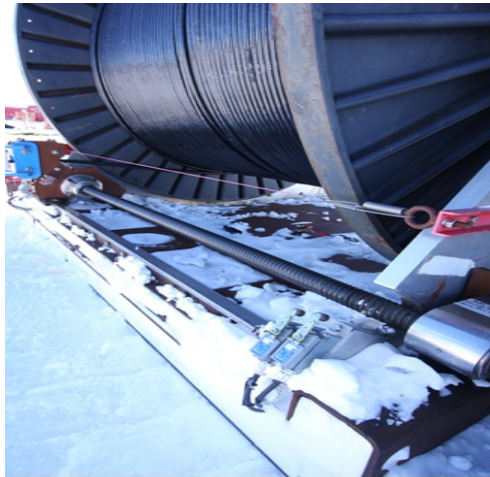
Figure 2.106 DCR level wind and safety E-stop trigger wire
