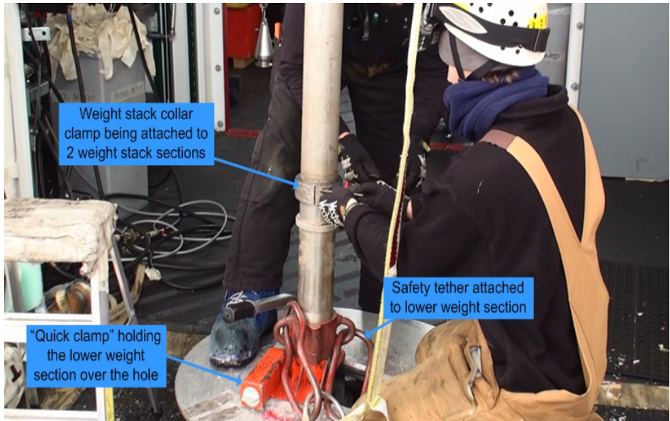
Figure 9.17 Weight stack collar clamp being attached to two weight sections.
