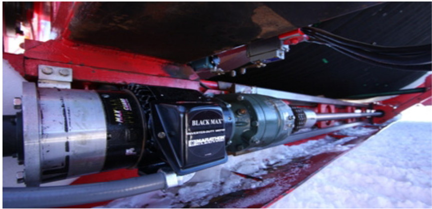
Figure 2.104 DSHR level wind system
