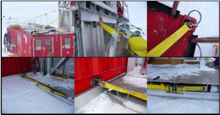
Figure 14.13 Securing tower to TOS using cargo straps and chains
