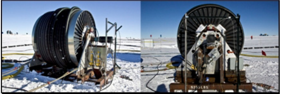
Figure 12.6 RWHR cable connectors (drum, brake and network cables)
